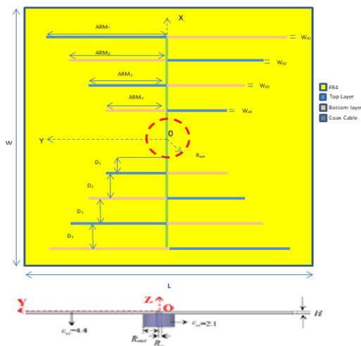
**Fig. 2.** Structure of Log Periodic Dipole Array Antenna.
