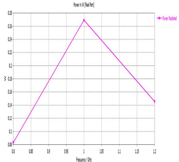
**Fig. 13.** Improved power radiated characteristics of modified design using CST simulator.
