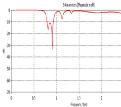
**Fig. 11.** The reflection coefficient of LPDA with modifications using CST simulator.
