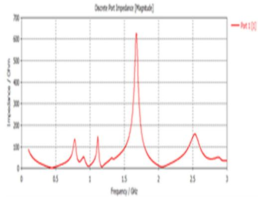
**Fig. 12.** Impedance characteristics of modified design using CST simulator.
